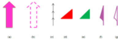
Figure 9.2 – Existing arrow types and approximate colours approved for use in ECDIS: (a) and (b) for traffic separation schemes, (c) for recommended (one-way) tracks, (d) and (e) for conical buoys,
