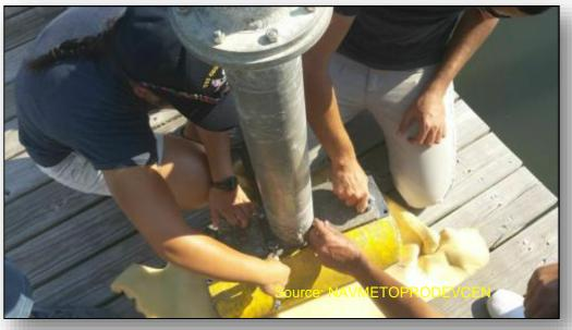
Installing a Multibeam Echosounder
