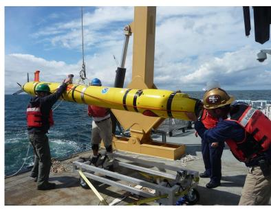
Deck and survey crew of the NOAA Ship Ferdinand R. Hassler deploy Coast Survey's Remus-600 bathymetric AUV in 2013 during the evaluation of AUVs for charting applications.
