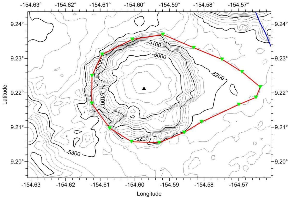
Fig. 3 Bathymetric and survey line map of the Yugong Hill (the contour interval is 20 m, blue ones are survey lines)
