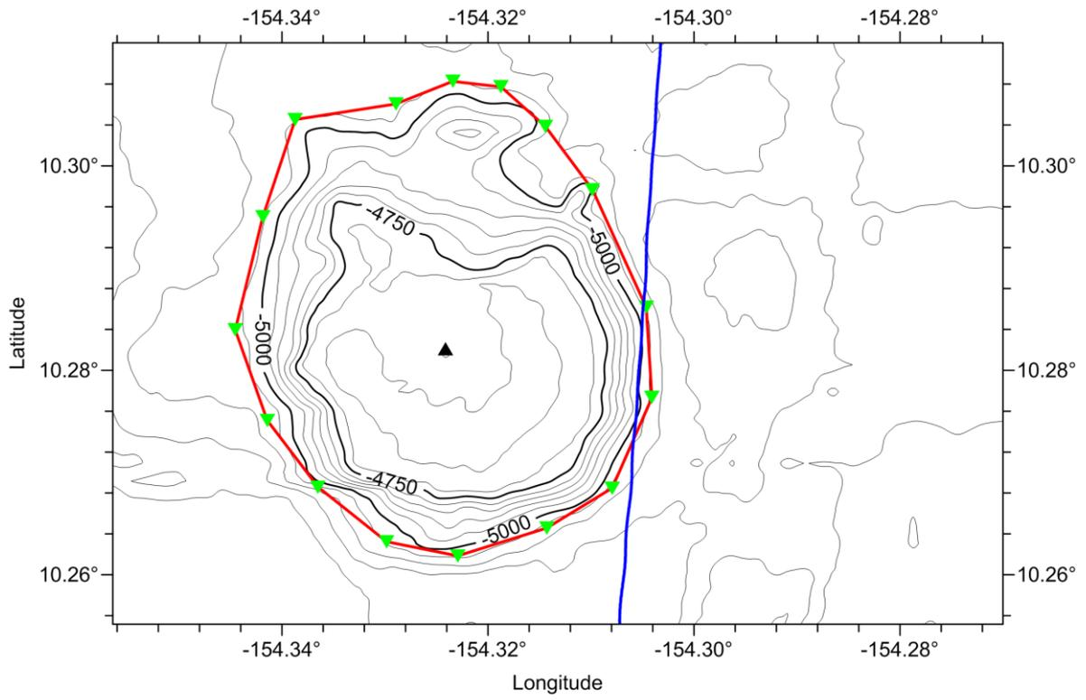
Fig. 3 Bathymetric and survey line map of the Jiefu Hill (the contour interval is 50 m, blue ones are survey lines)
