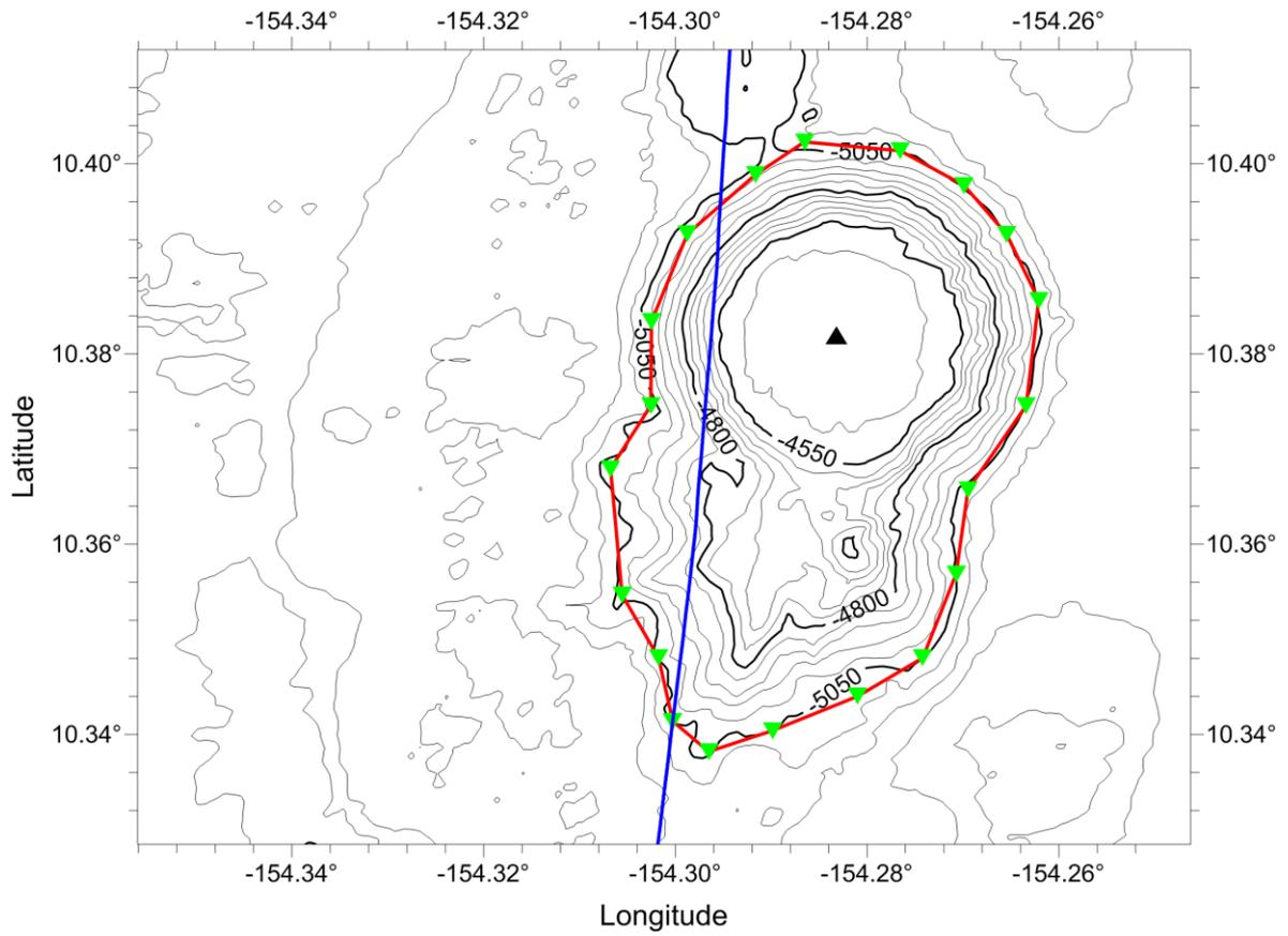
Fig. 3 Bathymetric and survey line map of the Shujun Hill (the contour interval is 50 m, blue ones are survey lines)
