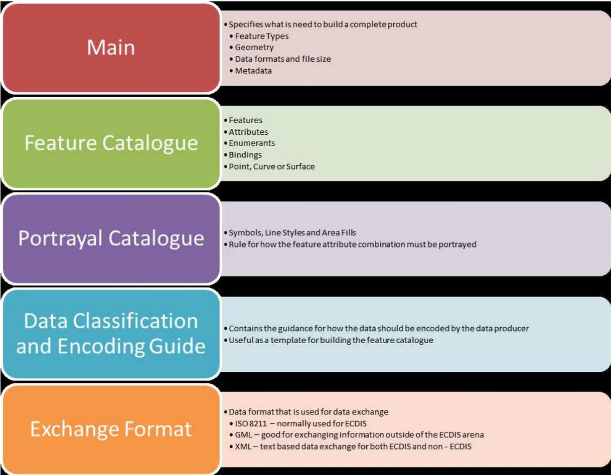
**Figure 2 - Structure of an S-100 based data product specification.**
