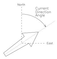
Figure 9.3 – Portrayal of the arrow's direction, based on the current direction. The dashed line is the arrow's centerline, and the origin of the East-North axis is at the arrow's pivot point.
