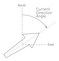
Figure J.2. Portrayal of the arrow's direction, based on the current direction. The dashed line is the arrow's centerline, and the origin of the East-North axis is at the arrow's pivot point.
