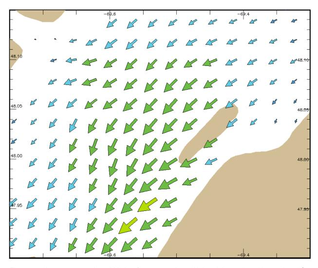
Figure 9.5 - Arrows representing gridded surface current data, with length increasing with speed, and S<sub>ref</sub> is 5 kn, H<sub>ref</sub> is 20 mm, and the maximum speed in the data in the image is 3.15 kn. Coastline added for clarity. Note that although some portions of the arrow symbol lie over land, the pivot point does not. (data courtesy of St. Lawrence Global Observatory, Canada)
