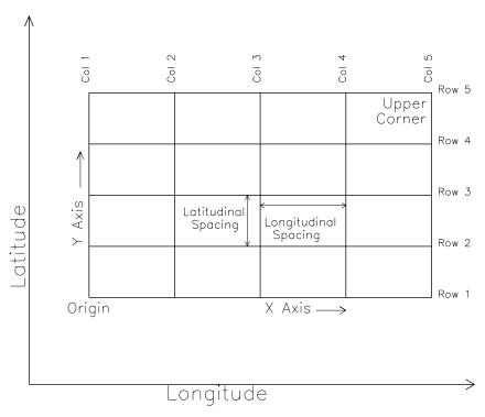
Figure 4.2 – Schematic of the regular grid and some of its attributes. The *offsetVectors* are shown as the Latitudinal Spacing and Longitudinal Spacing. The *origin* is shown at the lower left corner of the grid.
