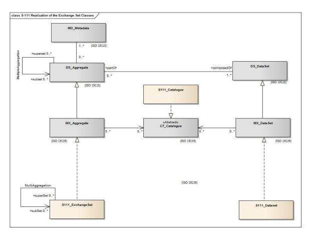
Figure 12.1 - Realization of the exchange set classes. Note that there are no support files.
