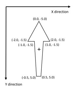
Figure J.1 - Surface current arrow symbol, showing x- and y-coordinates of the vertices (mm) and the pivot point (+).
