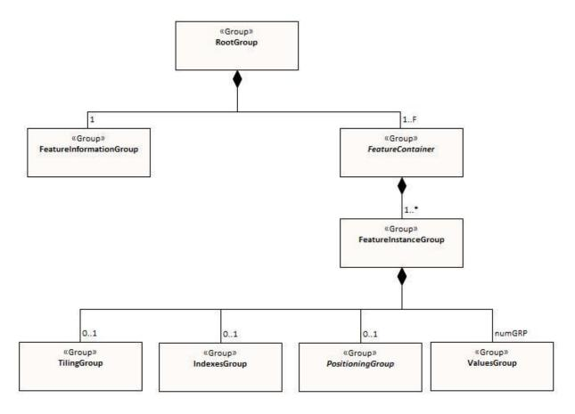
Figure 10.1 – Outline of the generic data file structure for all HDF5 formatted data files in S-100. (see Part 10c – Figure 10c-7)
