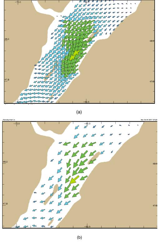
Figure 9.7 – (a) Surface current vectors (see Figure 9.6) displayed with identical parameters, but at low resolution. (b) Current vectors as in (a), but 'thinned' by plotting every fourth point. Note that the coastline data in the figure may differ from that used to determine model boundaries; in practice, the arrow pivot point must not be placed over land. (data courtesy of St. Lawrence Global Observatory, Canada).
