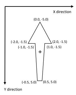
Figure 9.1 – Standard arrow symbol for use in representing surface currents. The coordinates of the vertices (x, y) are shown in mm. The '+' shows the location of the pivot point at (0.0, 0.0) and the y axis is pointing downward. Maximum height is 10 mm and maximum width is 4 mm.
