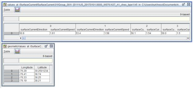
Figure G.2 – Compound array values for speed and direction in Group\_001 (top panel) and the longitudes and latitudes in the group Positioning (bottom panel).
