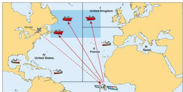
Figure 6 – SafetyNET message addressing to a rectangular area
