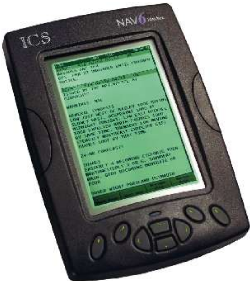
Figure 5 – Example of NAVTEX receiver with LCD screen
