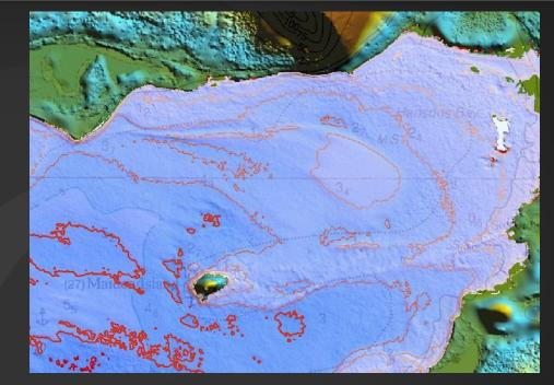
Using modern satellite imagery and physics-based SDB with stereo photogrammetric bathymetry validation, source bathymetry for Five Island Harbour was updated by ~170 years. Remote validation at +-12% of depth
