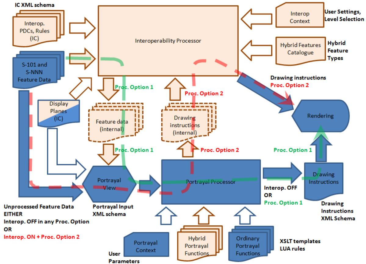
**Figure 6. Interoperability Processing Overview for Phase 2.**
