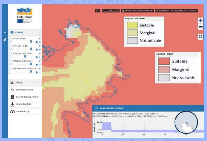
All Slovenian waters can be considered coastal. The area is rather small and shallow (average 17m). For this reason all the area should be covered with high resolution data. A 2 km buffer from coastline should be considered as priority area to be surveyed with high resolution data: approximately 92 km<sup>2</sup>.
