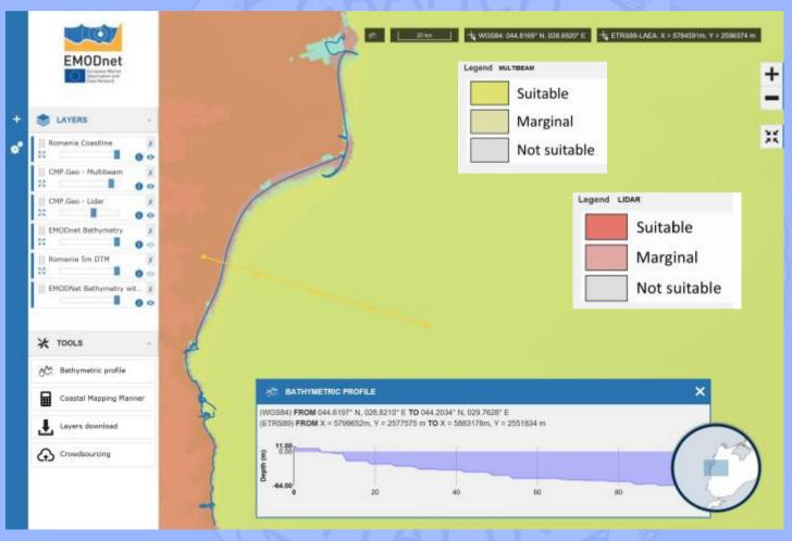
Enhance data density of 0-15m water depth region, but most probable it has to take into account an onshore buffer zone for Lidar surveying. GIS technology is used and the area to be covered is about 1500 km<sup>2</sup>.
