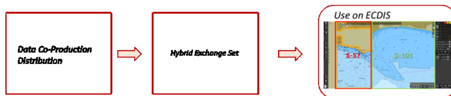
Figure 2: The physical data chain from production, packaging and use
