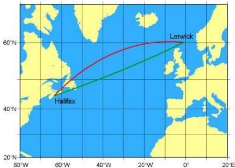
Figure 3. 9 - Part of the North Atlantic Ocean on the Mercator Projection, showing great circle (curved) and rhumb-line (straight) paths between Halifax and Lerwick
